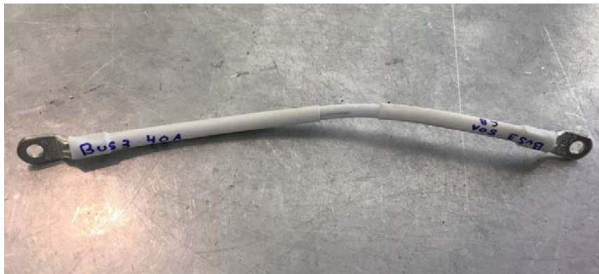
FIGURE 2 – Jumper Wire between 50 Amp and 40 Amp RCBs
