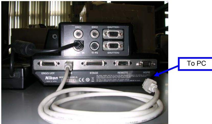
**Make sure the Hub is connected to the stand. It is unnecessary to disconnect any of the motorized components connected to the Hub.**
