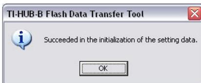
Click [×] on the upper right corner to end the HUB-B upgrade tool “HUB-B\_FDT.exe.”
