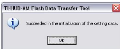
Click [x] on the upper right corner to end the HUB-A (main CPU) upgrade tool "HUB-AM\_FDT.exe."
