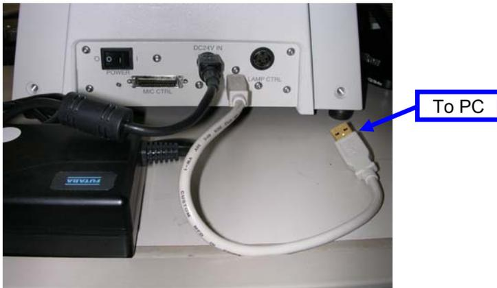
Connecting TI-HUBC/A Hub Controller A to the PC to upgrade Hub A or B firmware.
