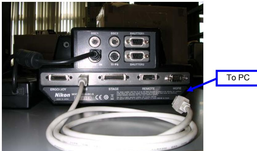
**Make sure the Hub is connected to the Ti-E stand. It is unnecessary to disconnect any of the motorized components connected to the Hub.**
