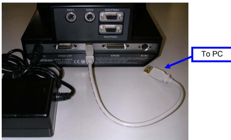
**Make sure the Hub is connected to the stand. It is unnecessary to disconnect any of the motorized components connected to the Hub**
